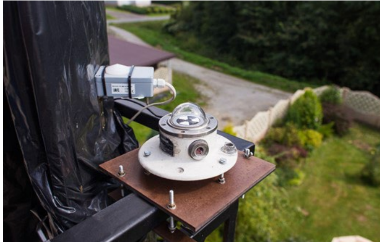
Fig. 4. Setting up the solar radiation meter in the building where the installation has been working Source: own study
