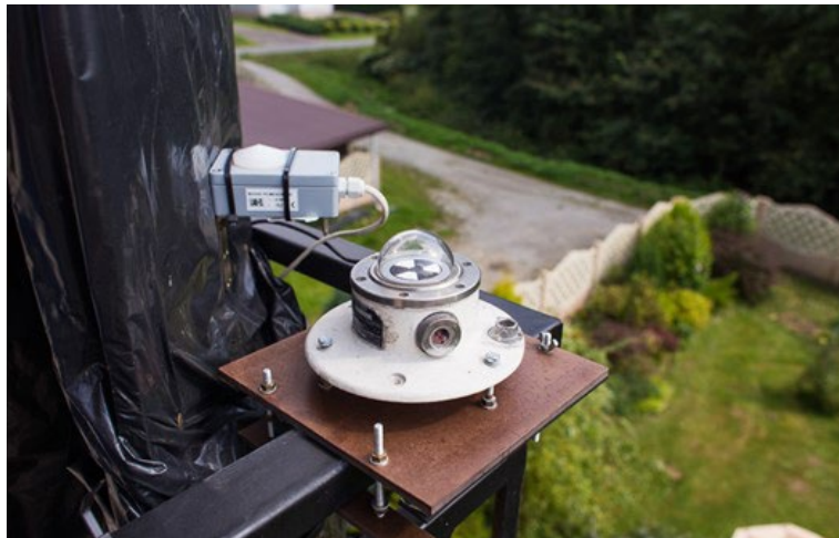
Fig. 4. Setting up the solar radiation meter in the building where the installation has been working
