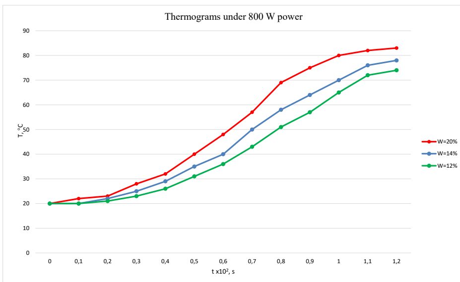
Fig. 2. Dynamics of heating rapeseed having different moisture content under the influence of electromagnetic emitter with 800 W power
