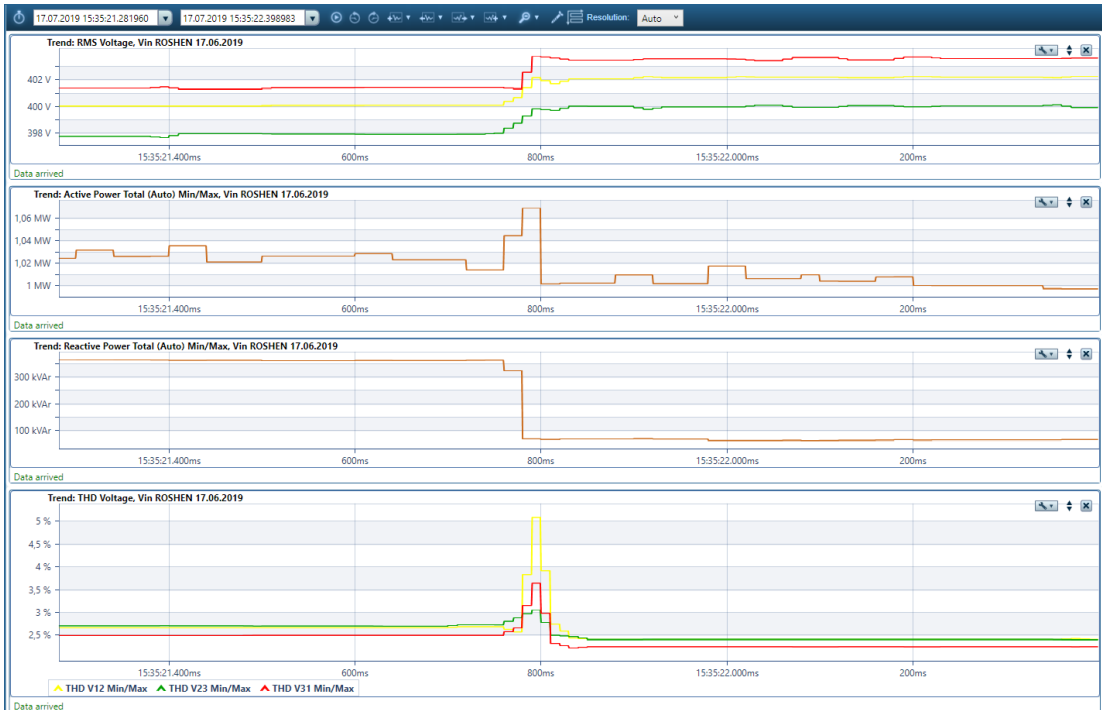
Fig. 17. Connecting a capacitor device with 189 Hz protective throttles
