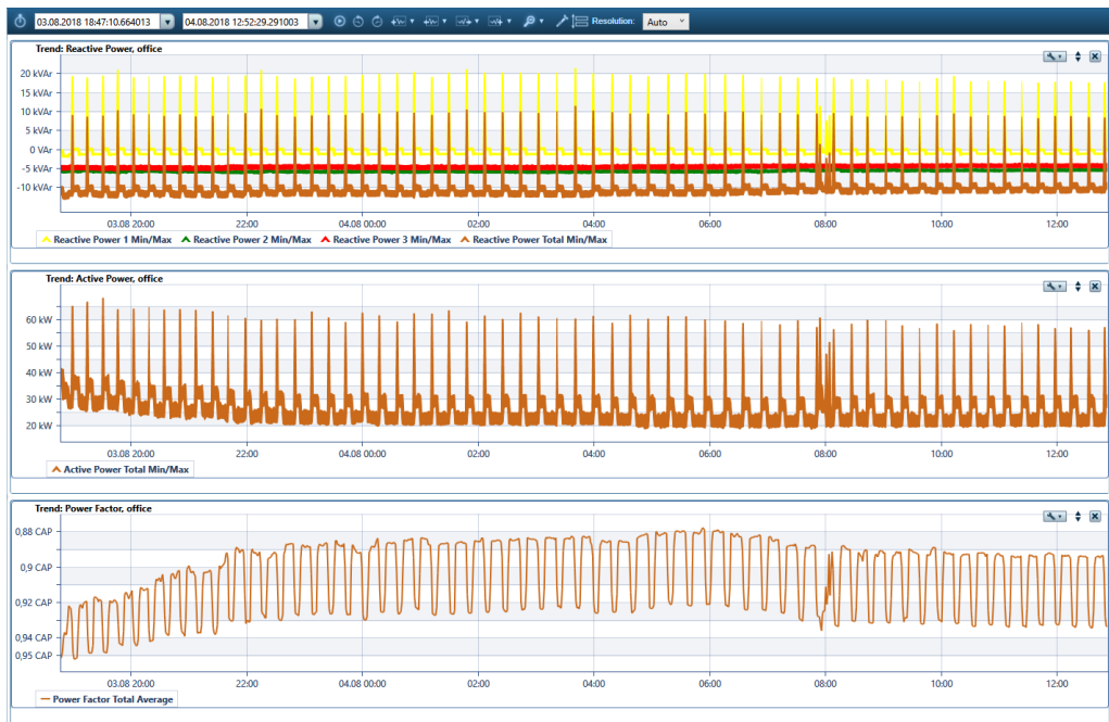
Fig. 6. Graphs of measurement of reactive, active power, and the power factor on the office power line
