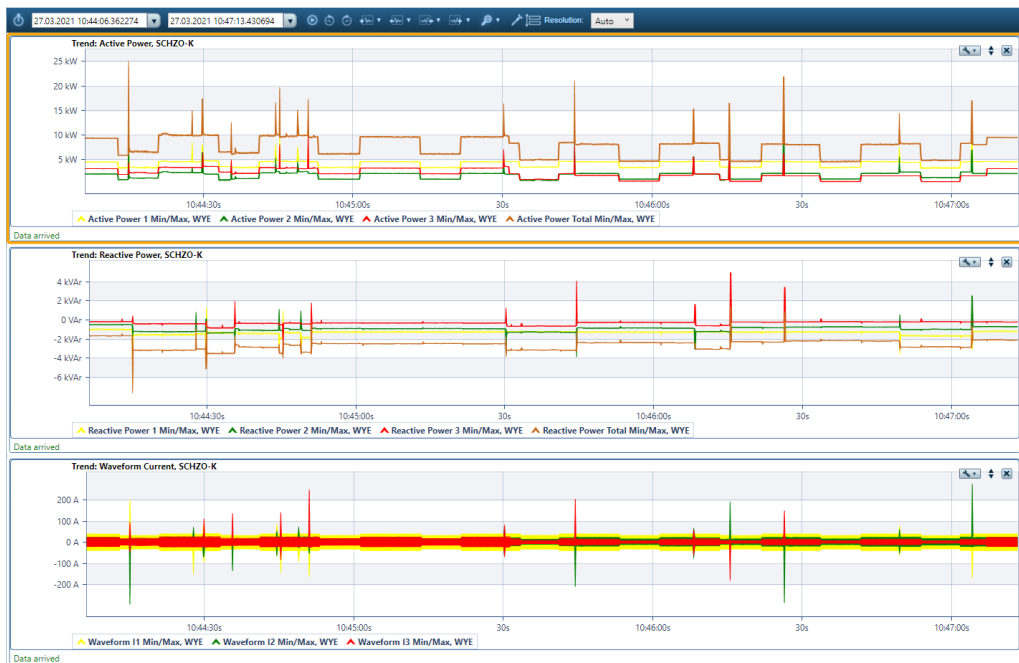
Fig. 5. Graphs of measurement of active, reactive power, and current waveform on the LED floodlight power line
