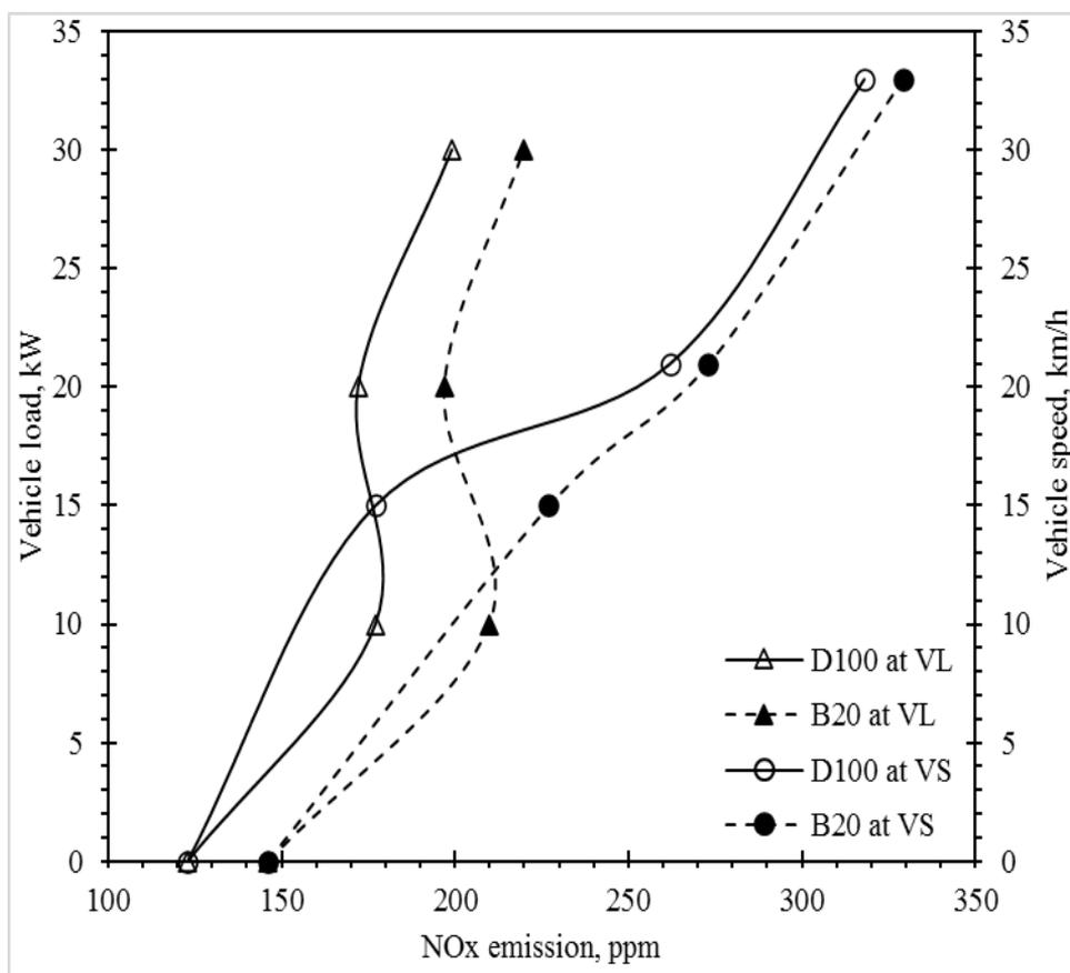
Fig. 9. NO<sub>x</sub> emissions of diesel and methyl ester-diesel mixtures at various vehicle speeds and loads
