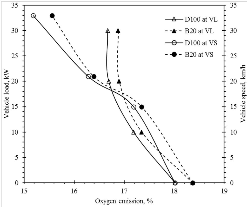
Fig. 10. Oxygen concentration of diesel and methyl ester mixtures at different vehicle loads and speeds
