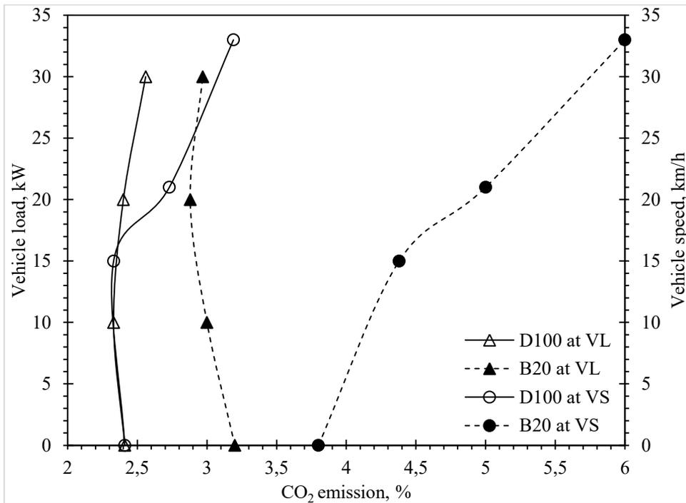
Fig. 7. CO<sub>2</sub> emission at different vehicle speeds for diesel and biodiesel blend
