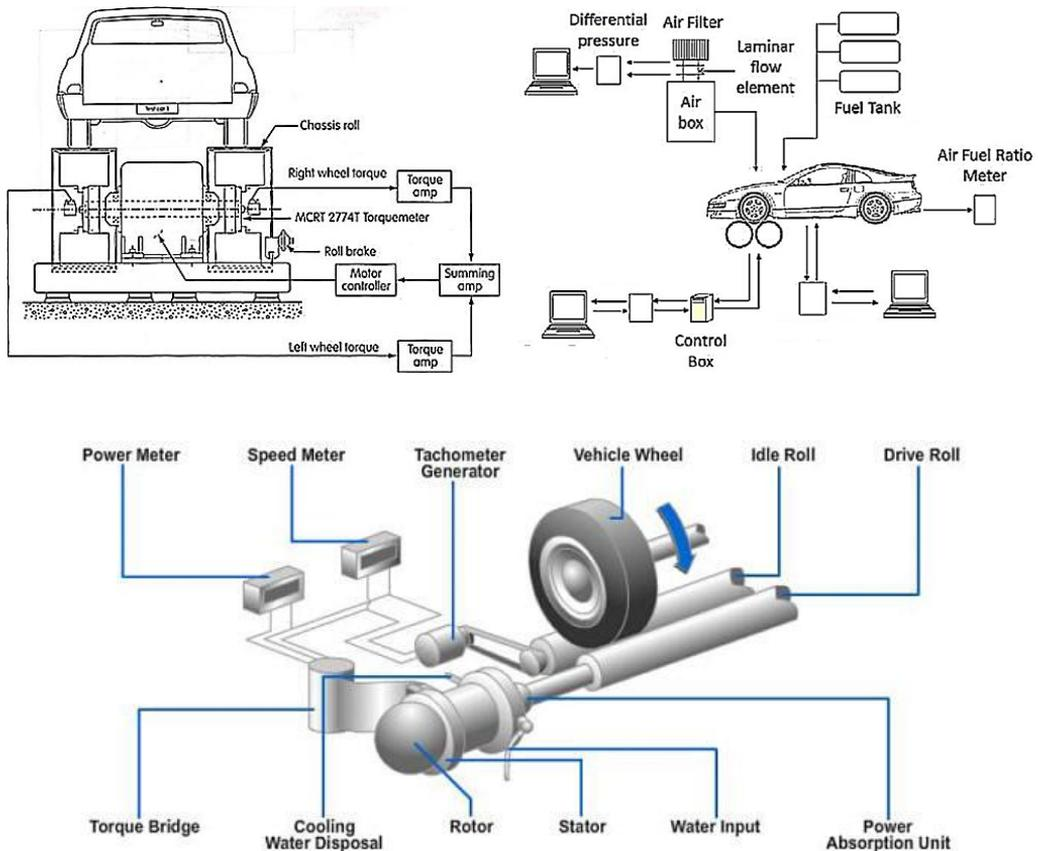
Fig. 2. Schematic diagram of the chassis dynamometer
