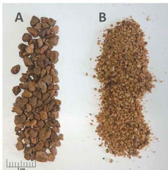
Fig. 2. A) Olive stones received for analysis. B) Olive stones after grinding in a knife mill to fractions smaller than 2 mm
