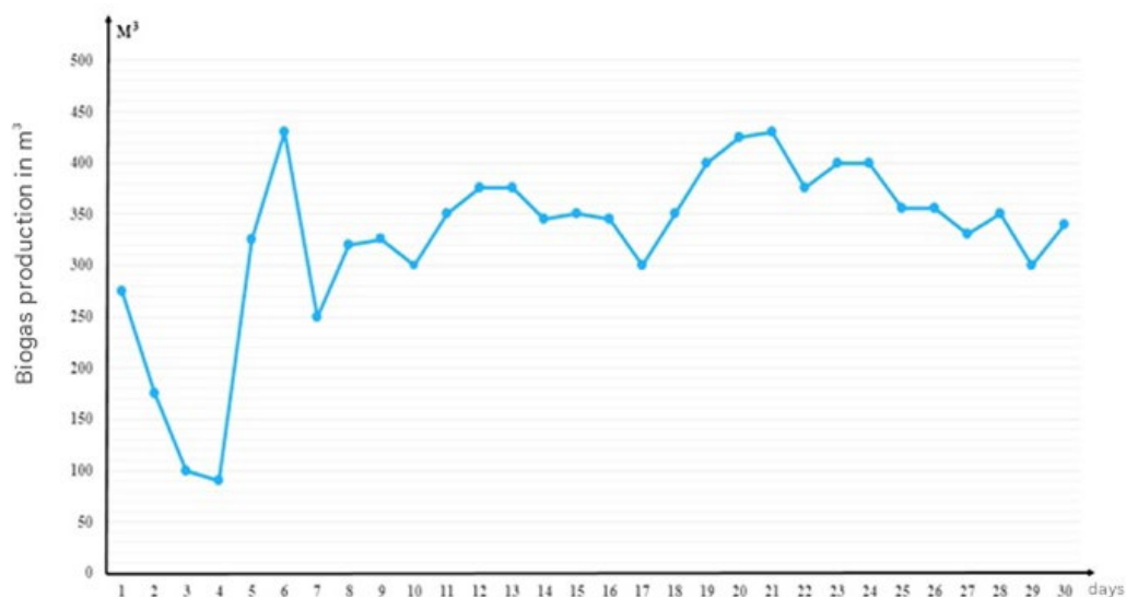
Fig. 1. Biogas production schedule with gradual loading of raw materials
