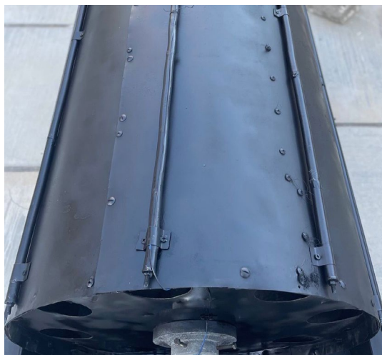
Fig. 1. A hollow reel with copper tubes fixed on it and painted with opaque black paint
