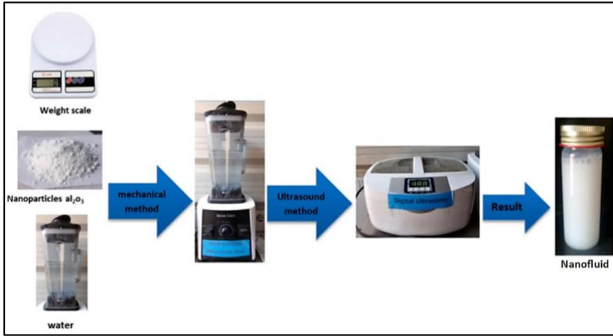
Fig. 3. Preparation steps of the \text{Al}_2\text{O}_3 /water nanofluid (magnetic stirring and ultrasonic dispersion)
