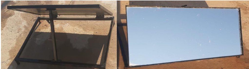
Fig. 2. The reflective mirror in the test system
