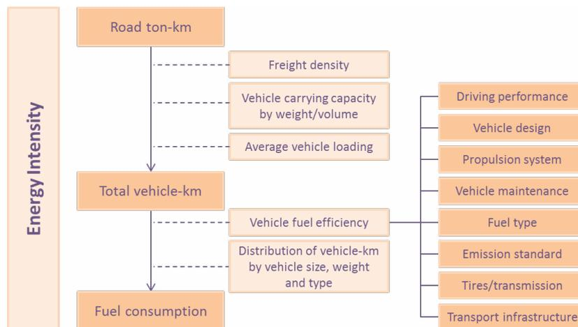
Fig. 24. Direct and indirect factors that affect the energy consumption in the road transport sector
